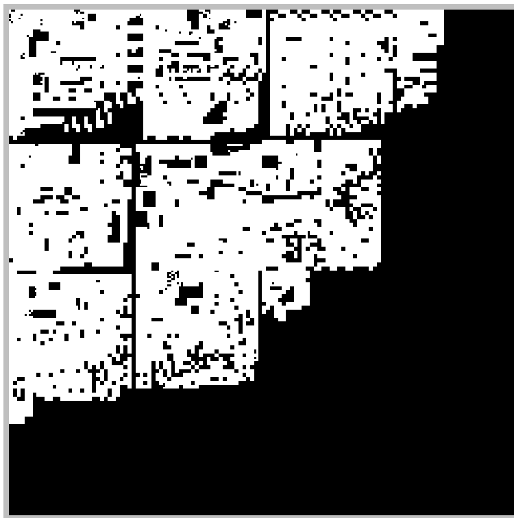
Figure 4.3: Flattened view of system illumination where white pixels represent an element that is non-zero at least once, and black pixels are always empty. The grey background was added to emphasise the borders and is not part of the texture.
